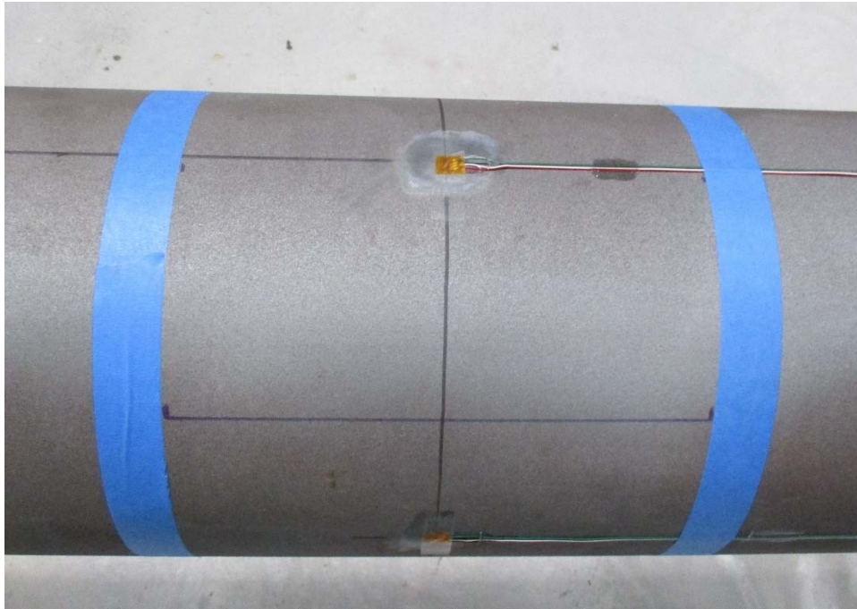
Image 2: Biaxial strain gages installed beneath the Effective Modulus Pipe Spring™ (Gages 1 through 4 in Table 2)
